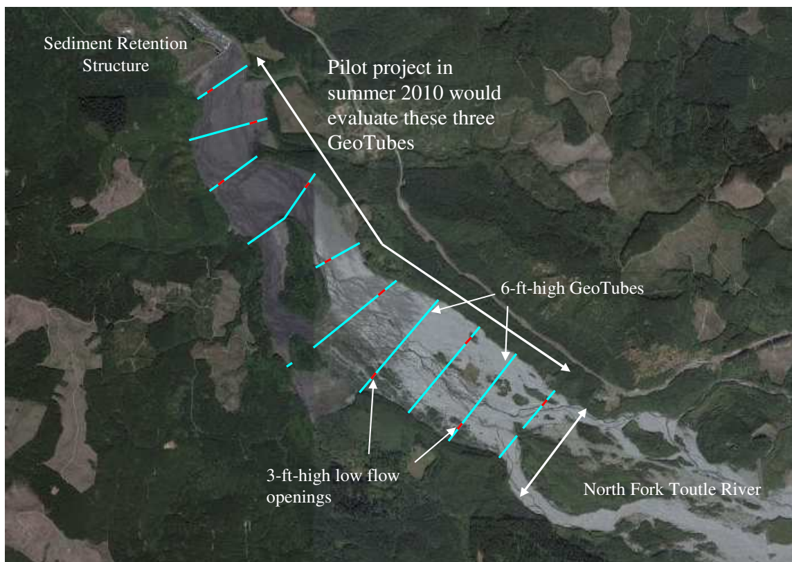
Figure 37 Possible deployment of low head sediment retaining dams using GeoTube Technology (Source: U.S. Army Corps of Engineers, Portland).
