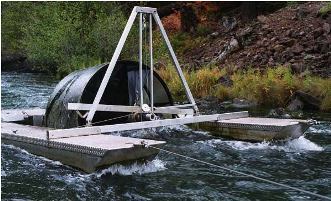
Figure 8. Intensive sampling of juveniles often relies on migrant trapping with a rotary screw trap. Where coupled with releases of mark groups to estimate trap efficiency, smolt trapping can provide estimates of absolute abundance of juveniles.
