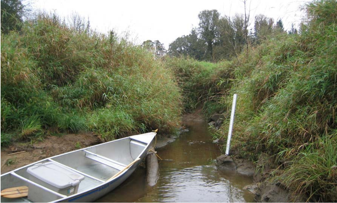
Figure 4. 65. Photo of mouth of McCormick Creek illustrating severe entrenchment and dominance of reed canary grass. Entrenchment here is approximately 1.7m. Entrenchment drops to 1.0m at the upper end of the survey.
