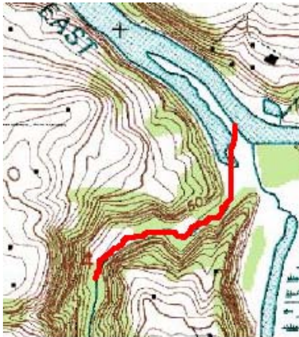
Figure 4. 58. USGS topographic map of McCormick Creek highlighting the stream survey area. Survey length is 0.9 kilometers. The stream channel no longer enters the East Fork Lewis as depicted by the USGS map, which shows the stream entering the large back channel. The highlighted survey area more accurately reflects the location of the stream, which bypasses the back channel and enters the main channel of the East Fork Lewis directly.
