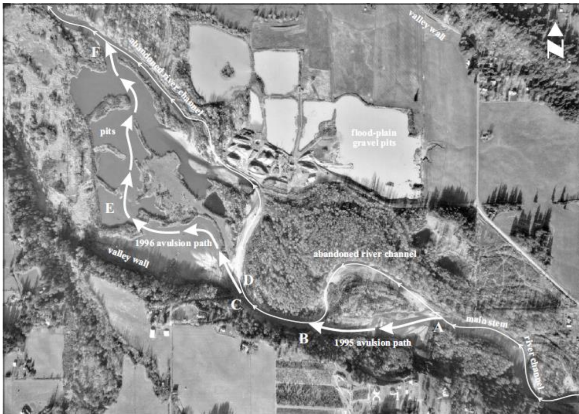
Figure 22. Figure from Flood Plains, Salmon Habitat, and Sand and Gravel Mining (Norman et al. 1998). The photo was taken in 1997 and shows the pathways of the 1995-1996 EFLR avulsions. Labels A, B, C, D, E, and F indicate locations where the river avulsed into the gravel pits, abandoned the historical channel, or re-entered its channel.
